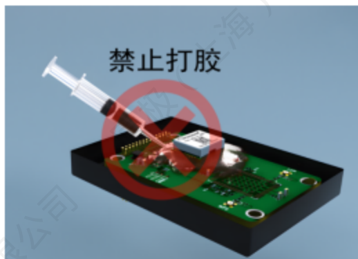
Figure 19 Schematic diagram of incorrect installation
