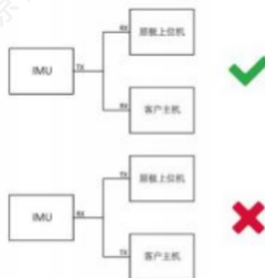
Figure 6 Schematic diagram of COM connection
