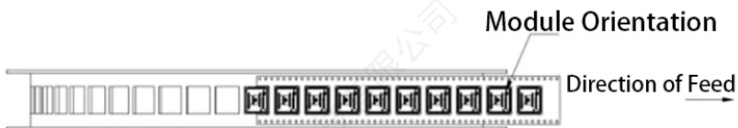
Fig. 16 Module Position and Orientation on Carrier Tape
