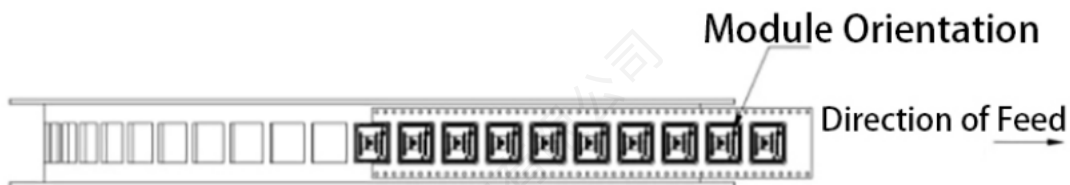
Fig. 30 Module Position and Orientation on Carrier Tape
