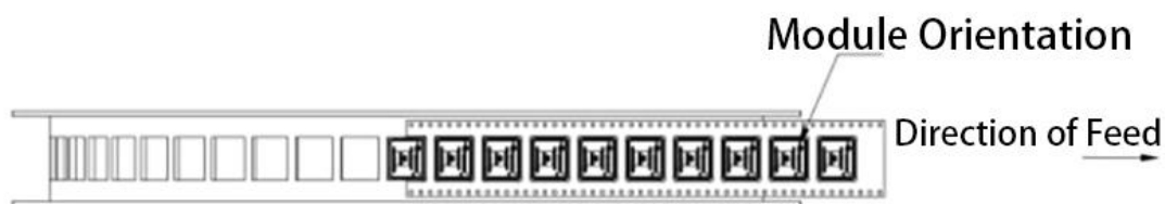
Fig. 26 Module Position and Orientation on Carrier Tape
