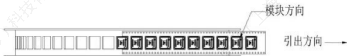
Figure 17 shows the position and orientation of the IMU614E-P
