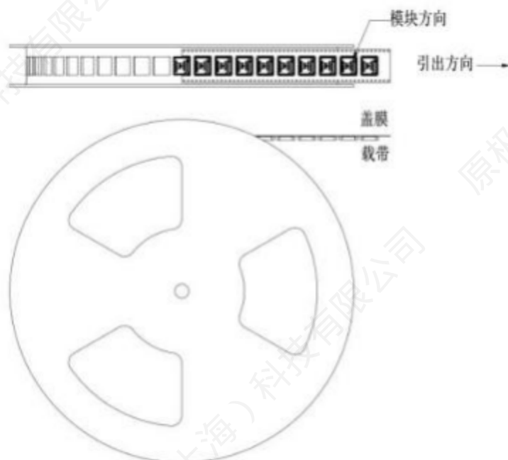
Figure 16 Schematic diagram of reel tape packaging
