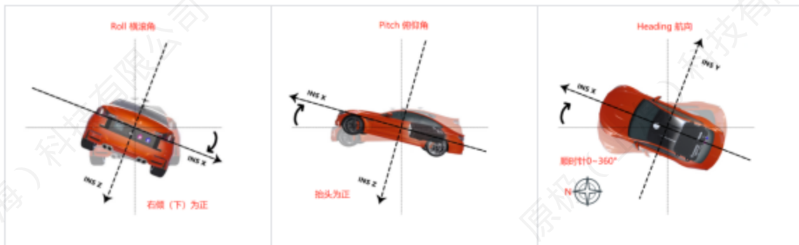
FIG. 21 Schematic diagram of roll, pitch and heading Angle
