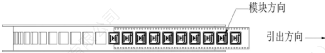
Figure 25 Position and direction of the IMU614E-Q on the load belt
