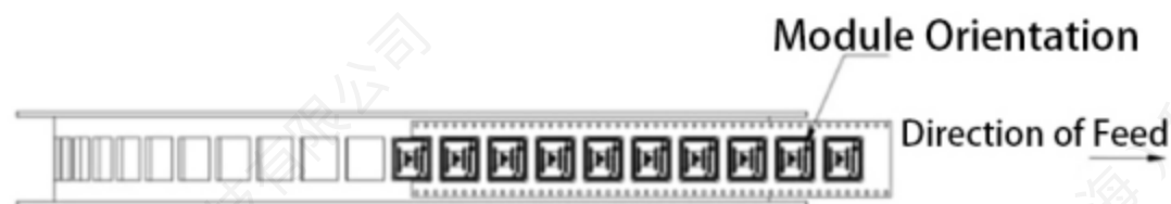
Figure 28 Position and direction of the IMU614E-T on the load belt
