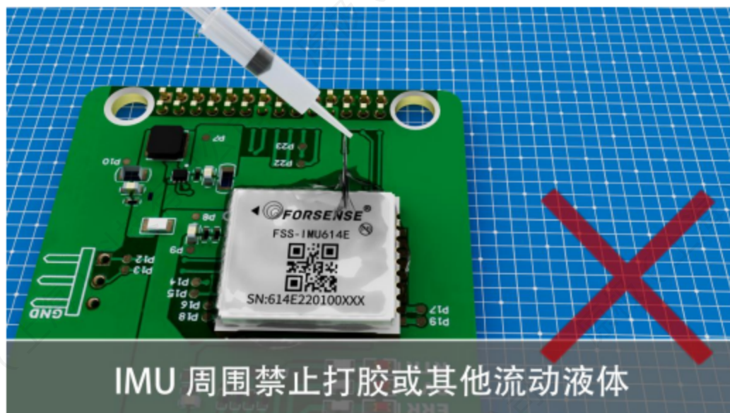
Figure 23 Schematic diagram of incorrect installation
