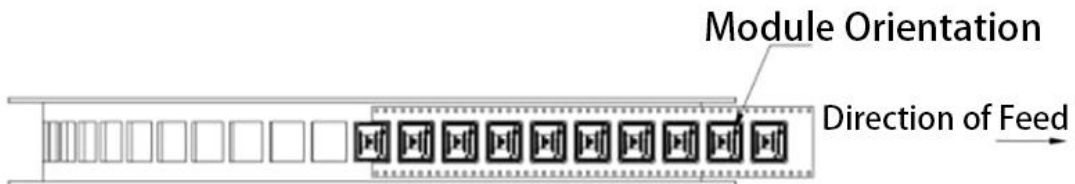
Fig. 30 Module Position and Orientation on Carrier Tape
