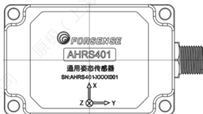
FIG. 8 AHRS401 coordinate system diagram
