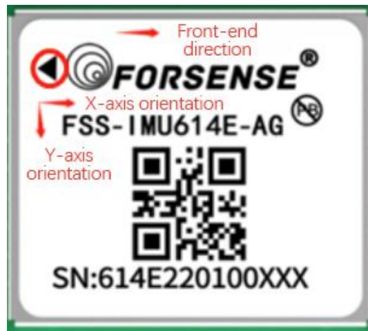
Fig. 7 Coordinate System Diagram
