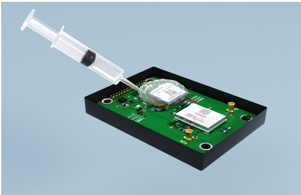
Fig. 22 Wrong Installation Diagram
