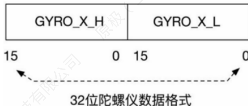
Figure 15 Schematic diagram of SPI32 bit data restoration
