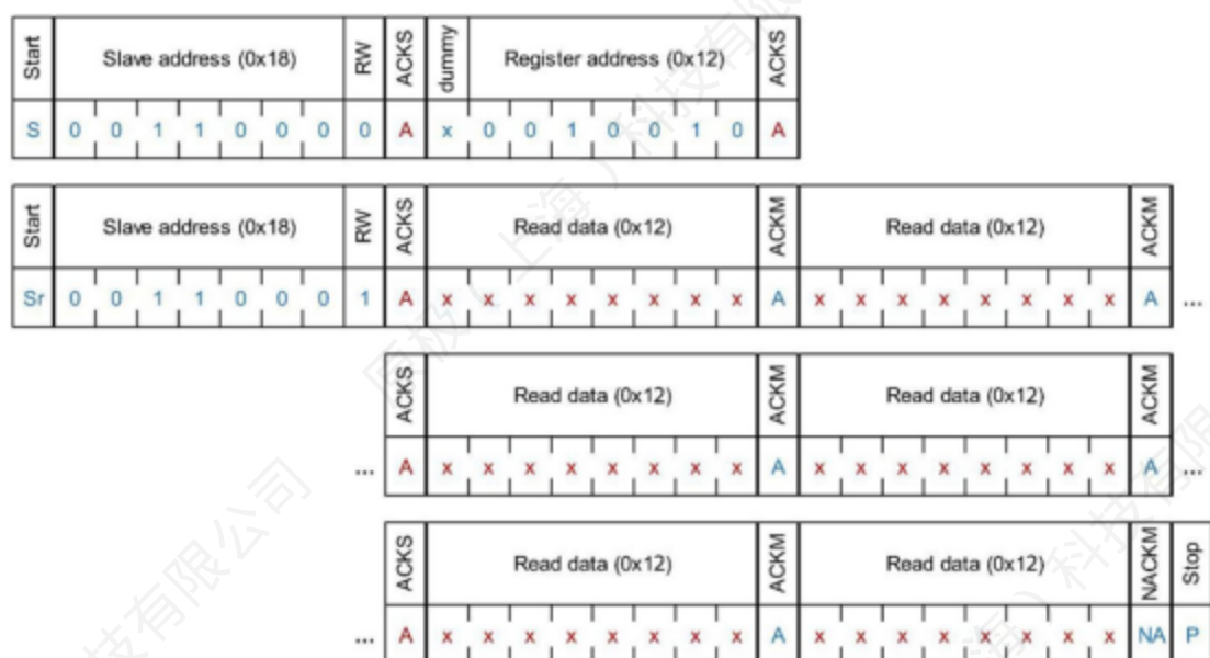
Figure 10 I2C continuous read mode
