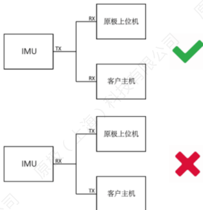
Figure 8 Schematic diagram of COM connection
