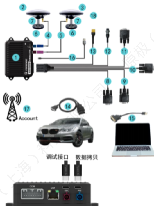
Figure 7 Physical connection diagram
