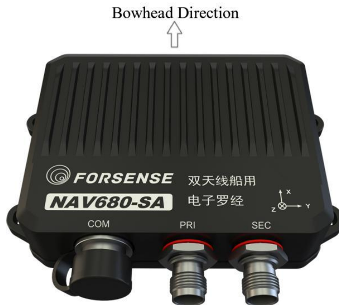
Fig. 5 Coordinate System Diagram
