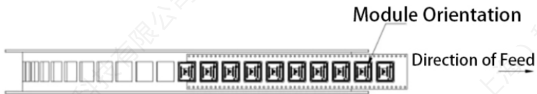
Fig. 8 Module Position and Orientation on Carrier Tape
