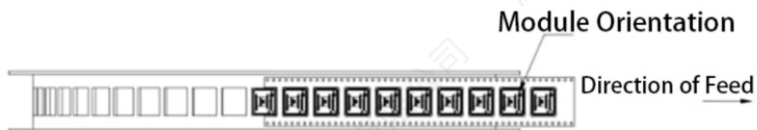
Fig. 8 Module Position and Orientation on Carrier Tape
