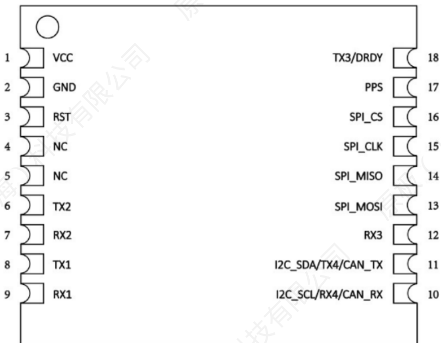
IMU614E-X Pin Layout (Top View)
